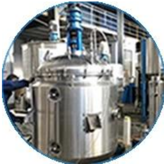
Layin injin cream
