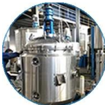
Layin injin cream
