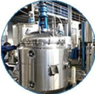
Layin injin cream
